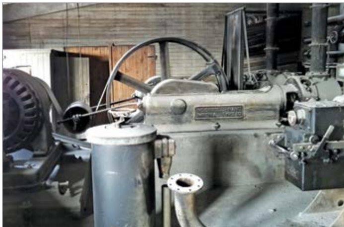
Paul Edwards discovered this Imperial Type 10 air compressor at a plant in Finland, where it performed for over 90 years. He believes there will be as much change in the compressed air industry in the next 20 years as there has been since this model was built.
